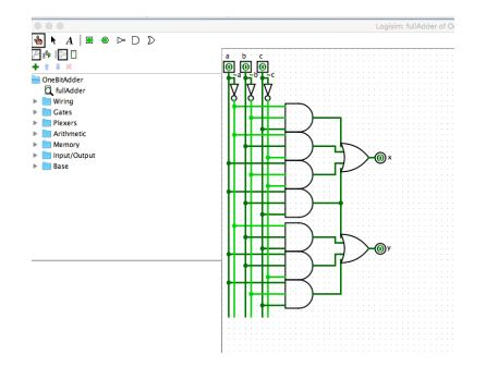
Edit its chip as shown bellow: <u>a</u> is one input (used to be <u>x</u>), <u>b</u> is the other input (used to be y), <u>c</u> input is the <u>carry in</u>, <u>y</u> output is the <u>carry out</u>, <u>x</u> output is the <u>sum</u>. Make the chip 4 pixels width and 5 pixels height as shown below.
